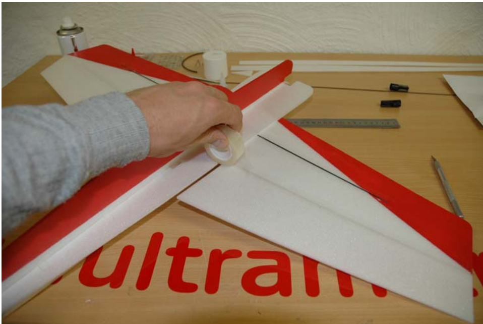
Hengse det andre roret. Hing the last aileron with clear tape.
