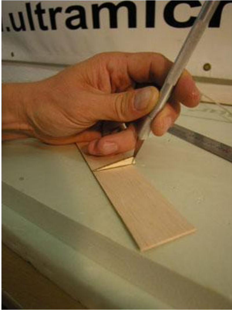
Kutt balaserorets ribber i en svak vinkel. Cut aileron ribs angled.
